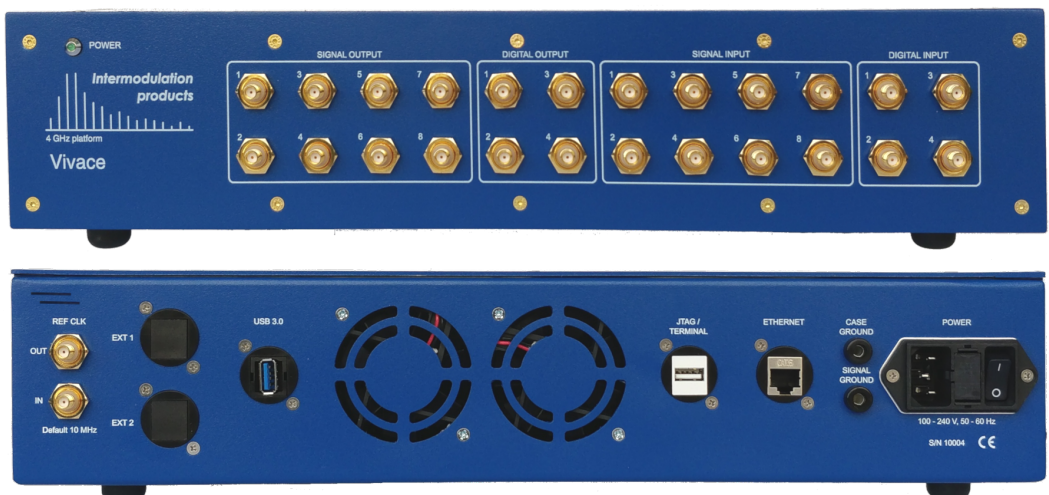
Figure 4: The front and back panel showing Vivace's connections: 8 input and 8 output signal ports (14 bit resolution), 4 input and 4 output ports for digital triggers or markers, clock reference for synchronization to external instruments, and ethernet connection for data transfer. A specification sheet is found here .
